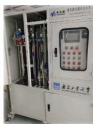
2 tons/day Spiral-wound NF Equipment
