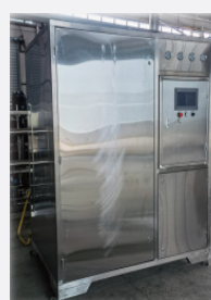
5 tons/day anodizing acid recovery unit
