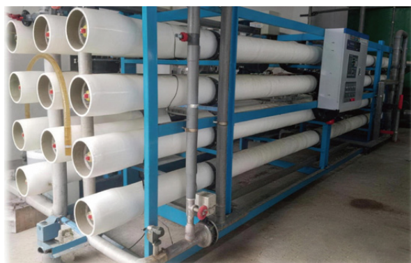
Zero-liquid Discharge Demonstration Unit for Sodium Acetate Wastewater
