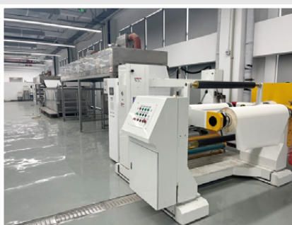
Flat Membrane Coating Line
