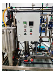
3 tons/day Hollow Fiber NF Equipment
